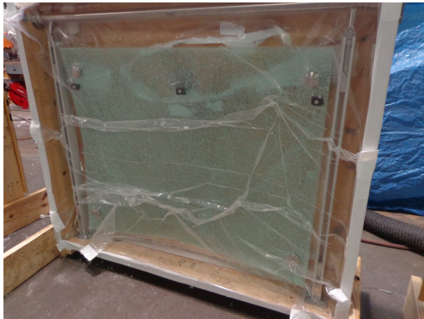
Photo No. 3 Typical Set-up for Pressure Applied to Filmed Side of Specimen
