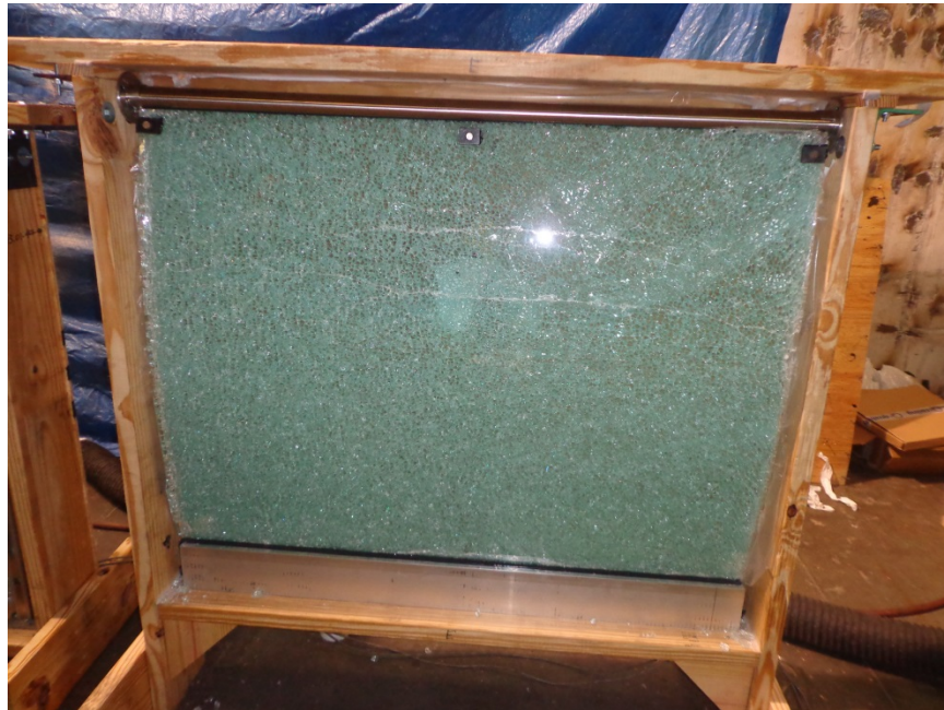
Photo No. 2 Typical Set-up for Pressure Applied to Non-filmed Side of Specimen
