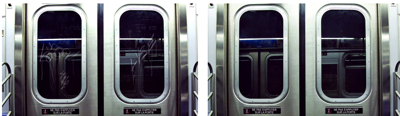
Glass protected by Graffitigard which has been tagged.
