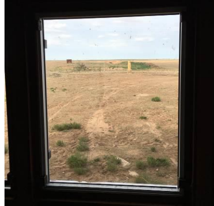
Figure C.20: Specimen 2-2 Pre-Blast Condition Interior
