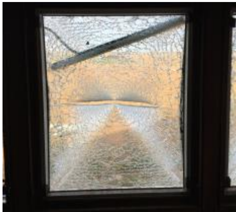
Figure C.27: Specimen 2-3 Post-Blast Condition
