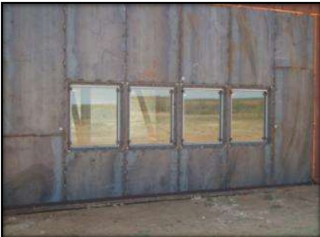
Figure B.3: Pre-Blast Specimen Setup Chamber 3
